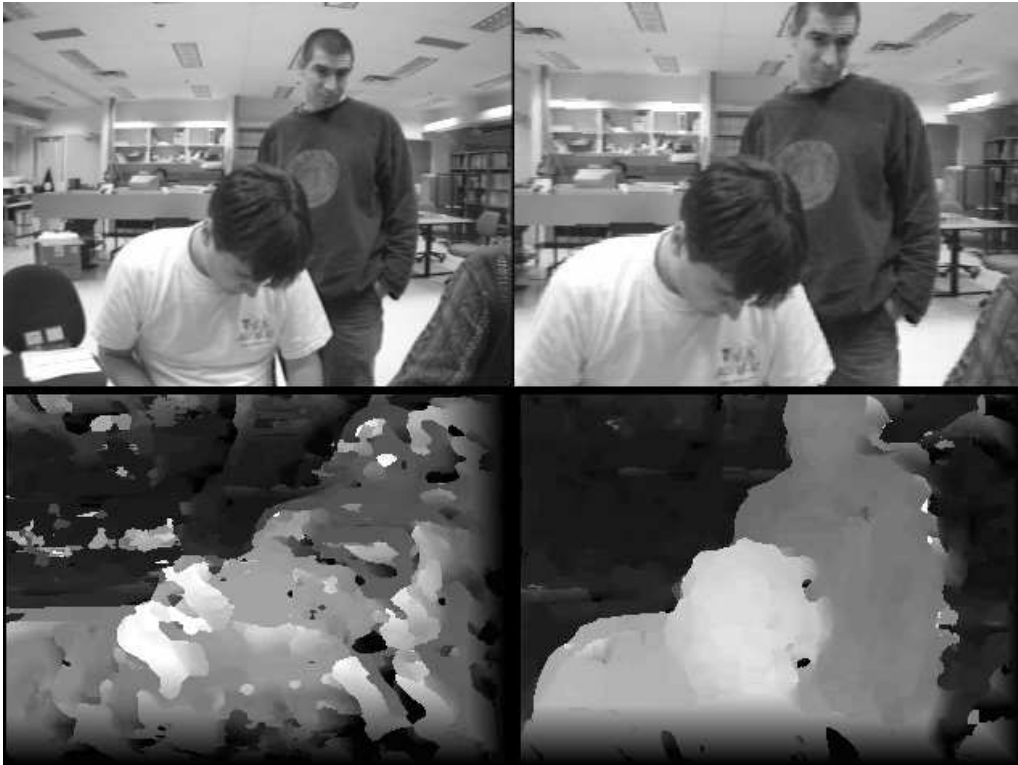
Figure 2.6: The left pictures demonstrate stereo results with radially distorted input images. On the right, the effect was corrected prior to the calculation [9].
